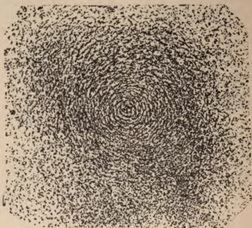
FIG. 35.—Concentric circles of magnetic force around a "live," or current-bearing, wire.
